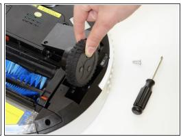
The left and right wheels are held on bObi with two screws. Uninstall them from the wheel you're replacing, and flip bObi over.
