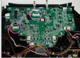
Detach the two circuit plugs connecting bObi's cover to the main board and the cover will be completely removed.
