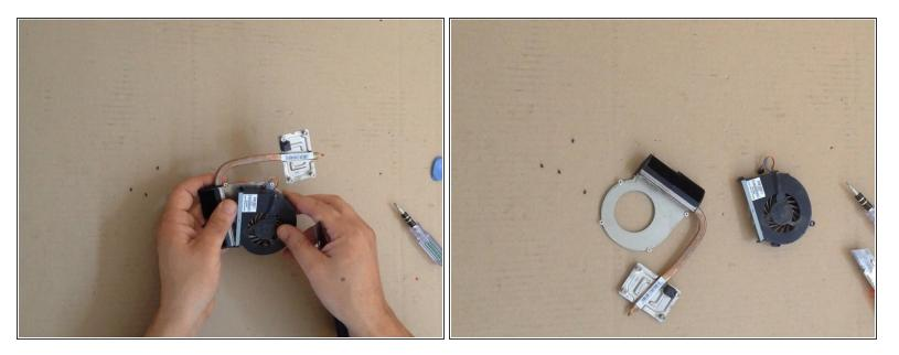
• Open the fan and clean the dust from inside with a soft brush.
