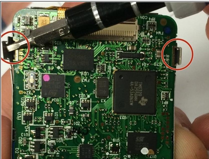
**!** Be gentle when removing the main board. The main board is attached to the front panel of the device by wires.
