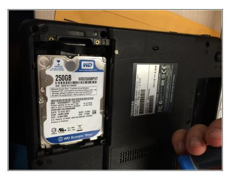
Pry up the cover of the hard drive compartment.
