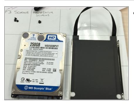
Remove hard drive from the casing by gently sliding the drive out of the case.
