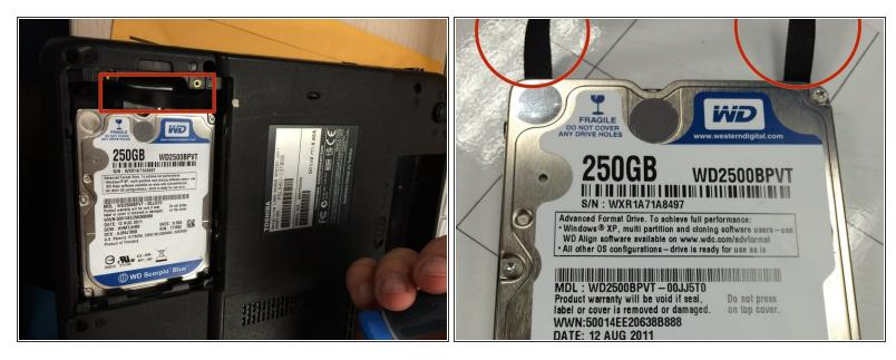
Slide hard drive out by pulling gently on the felt handle
