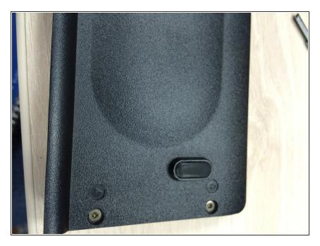
Remove the two screws marked "4" from the hard drive cover
