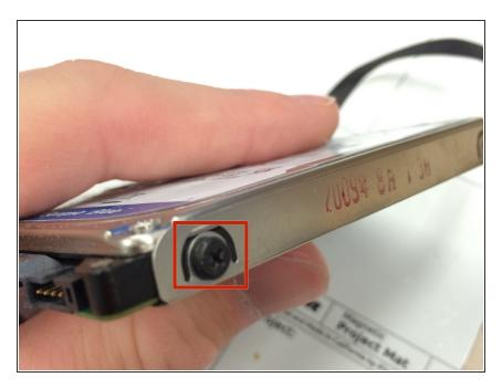
Remove four outer black screws on the corners of the hard drive case
