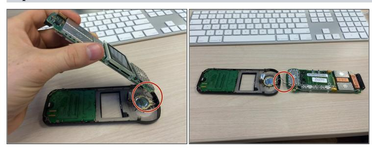
• Flip the motherboard over so that the screen is facing down.
