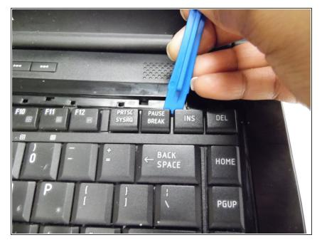
Use plastic opening tool to pry out the keyboard, starting by the 'delete' key in the top right corner.
