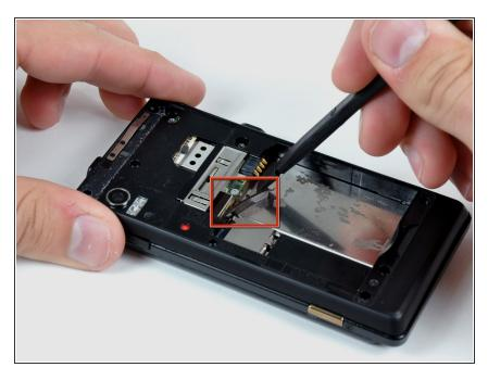
Insert the flat end of a spudger and pry downwards to release the plastic tab holding the rear case to the motherboard screw.
