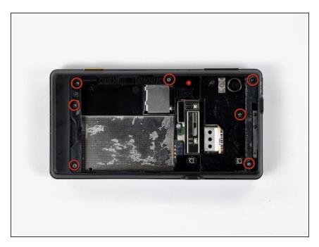
Remove the seven 5.5 mm T5 Torx screws securing the rear case to the inner case.
