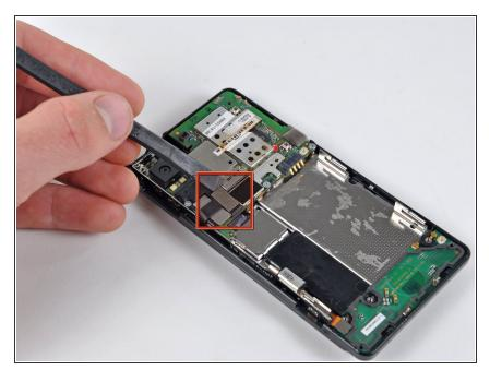
Disconnect the power button/volume button connector from its socket on the motherboard using the flat end of a spudger.
