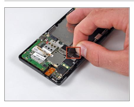
Peel the black tape covering the side button and display ribbon connectors on the motherboard.
