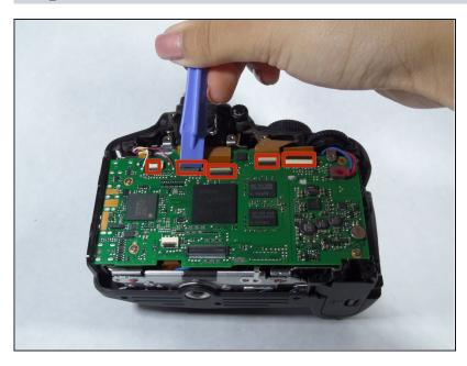
Carefully flip the 5 brown plastic connectors using the plastic opening tool.
