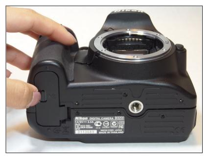
Find the marked arrow on the battery compartment door and firmly push following the arrow's direction to release the latch.
