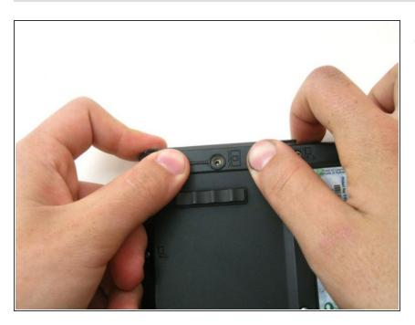
• Pull the hard drive out with of its bay the help of pictured ridges. Carefully remove it.
