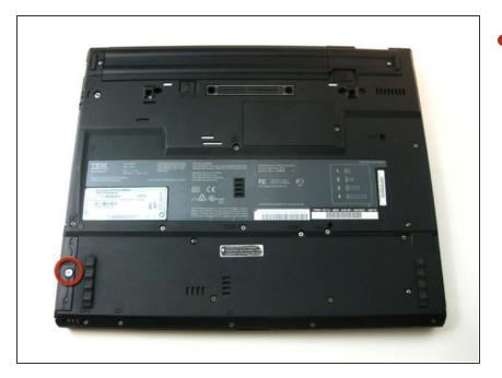
• Unscrew the single screw holding the drive cage in place.
