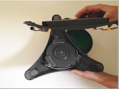
Gently lift and separate the back housing from the rest of the device. Now you've got the back housing off!
