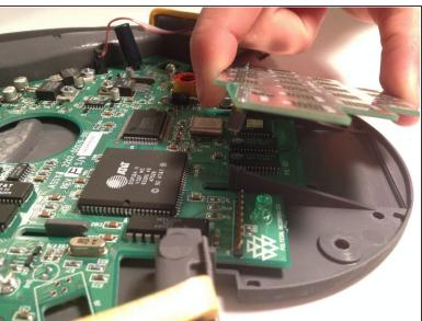
Gently lift the internal keyboard off of the motherboard.
