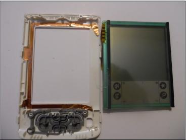
Carefully, remove the screen from the device by lifting up and replacing with a new one.
