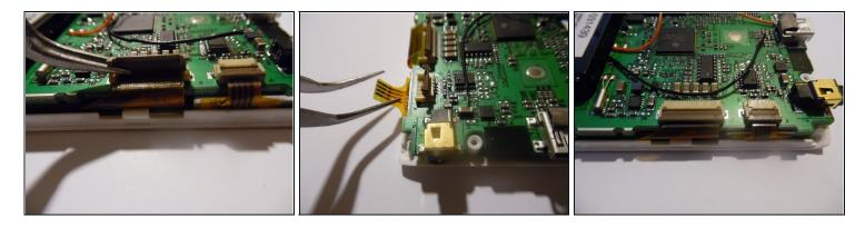
• Using <u>tweezers</u>, or something similar flip up the tab, releasing the wires located under the flap
