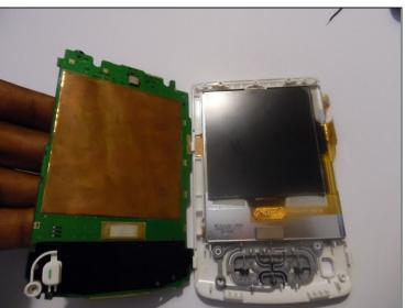
• Gently, remove the motherboard by lifting up exposing the screen.
