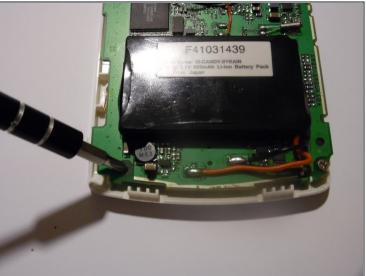
• Using a Philips head screwdriver, remove the two screws located at the bottom of the board.
