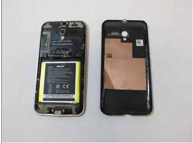
Use plastic opening tool to pry off the back cover of the phone.
