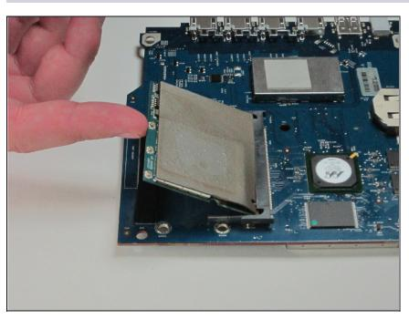
After holding back the plastic piece keeping the card in place, lift the card up and pull it away from the logic board.
