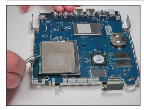
• Unhook the wires connecting the logic board to the metal casing by grabbing and pulling up on each connection with tweezers.
