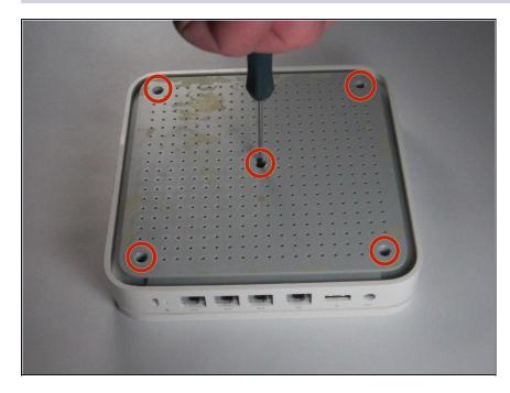
After removing the rubber pad, unscrew the five 5mm phillips #00 screws in the holes of the back cover.
