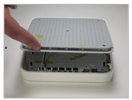
Lift up the back case from the perforated edge to remove it.
