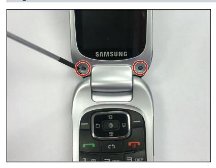
Loosen the screws under the soft screw covers using a Phillips #00 screwdriver.
