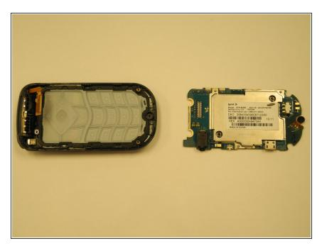
If intending to reuse the logic board, be sure to place it in a space that minimizes contact with dust and dirt.
