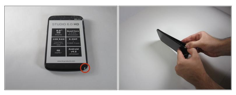
• To begin the removal of your back panel, first locate the lift tab on the bottom-right corner.
