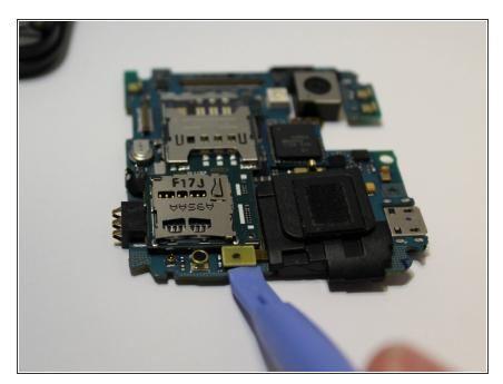
Using the plastic opening tool, detach the tab connecting the speaker to the motherboard.
