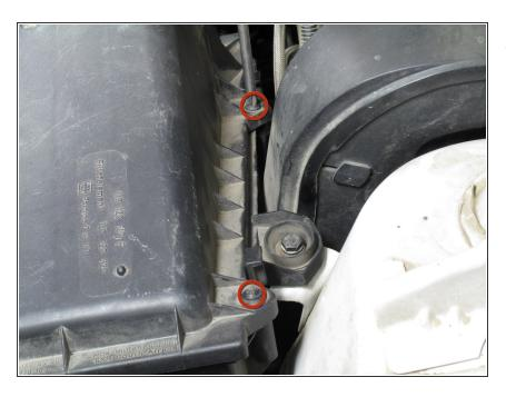
Unscrew two Phillips screws located behind the air filter.
