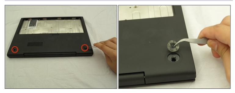
• Using a pair of <u>tweezers</u>, remove the two rear rubber feet to expose two hidden screws.
