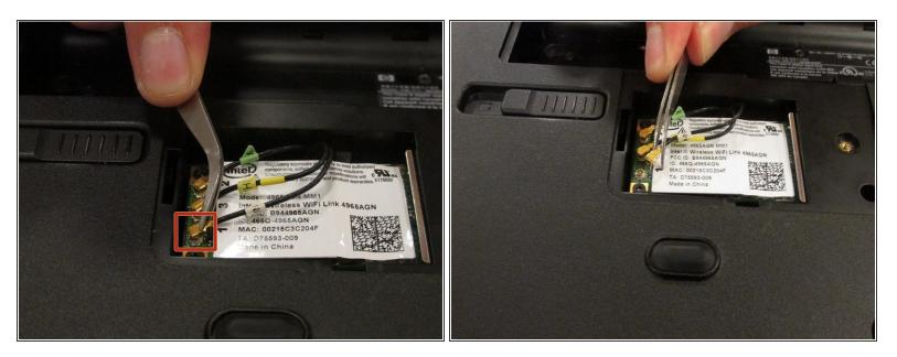
• Use a pair of tweezers to remove the three antennas from their sockets.
