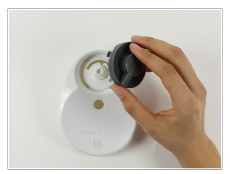
Fully remove the dial by pulling it out from the front.
