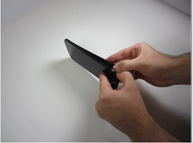
• To begin the removal of your back panel, first locate the lift tab on the bottom-right corner.
