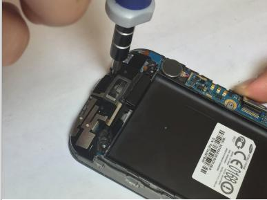
Unscrew 4.4mm with a PH #000 marked screw.
