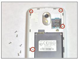
Remove 4.4 mm screws using a PH # 000 as indicated on the picture.
