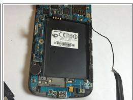
Remove the antenna using either your fingers or tweezers.
