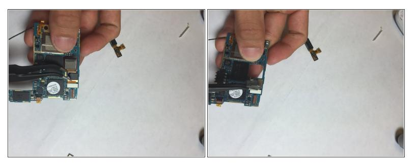
Using tweezers pull out the back camera lens from the circuit board.
