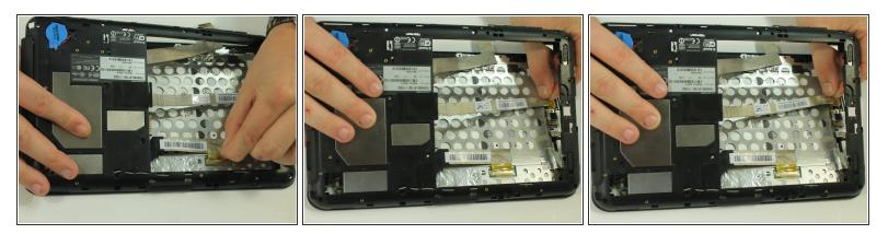
Once the back of the case is off, disconnect the wires by gently pulling on the plastic tabs as shown.
