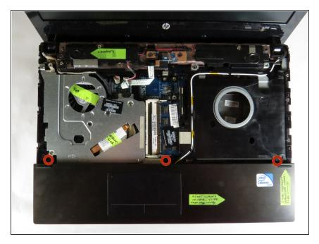
Unscrew the three (2.5 mm Phillips) screws holding the bottom touchpad panel.
