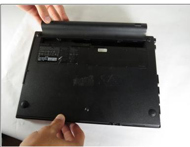
Flip the laptop upside down and remove battery by pressing inward on the two latches holding the battery in.
