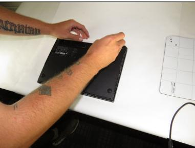
Unscrew the four (2.5 mm Phillips) screws (Use Phillips #0 Screwdriver).
