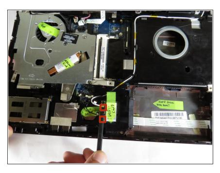
Using the black spudger, detach the two antenna cable connectors
