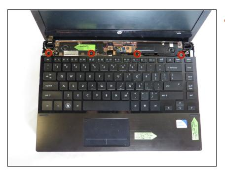
Unscrew the four (2.5 mm Phillips) screws holding the keyboard in (Use Phillips #0 Screwdriver).
