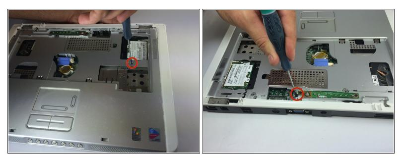
Remove two 4 mm Philips #00 screws that connect top of laptop to base..
