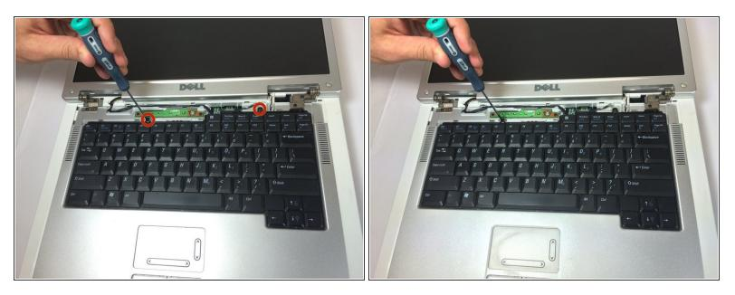
• Remove two 4 mm Philips #00 screws.
