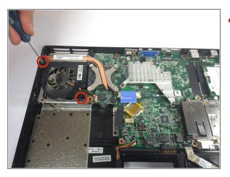
Remove two 4 mm Philips #00 screws.
