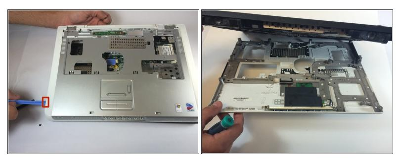
Insert the plastic opening tool in between the back and front plates of the laptop
