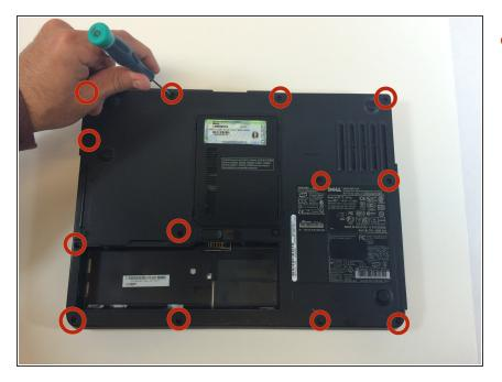
• Flip laptop the over and remove thirteen 6mm Philips #00 screws.
