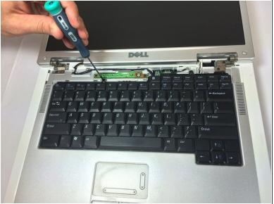
Remove two 4 mm Philips #00 screws.
