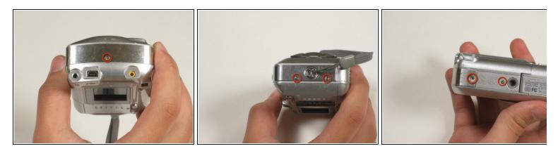
• Remove five screws from the camera casing using a tri-point Y0 screwdriver.
