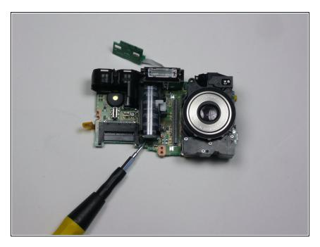
Locate the flash unit of the camera. It includes the camera's flash and a capacitor.
