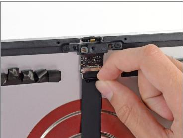
• Flip down the metal retaining bracket on the iSight camera cable.
