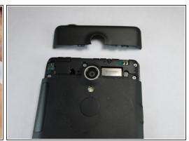
Use the plastic opening tool to pry the top plastic section off.
