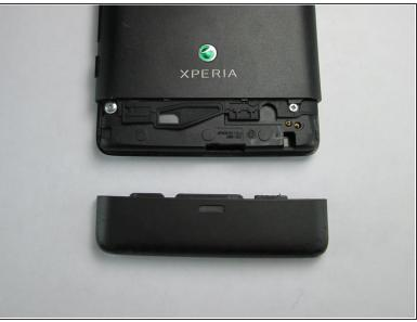
Use the plastic opening tool to pry the bottom plastic section off.
