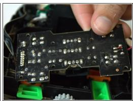
Remove the eight black 7.2 mm Phillips #0 screws from the top of the circuit board and remove the circuit board.
