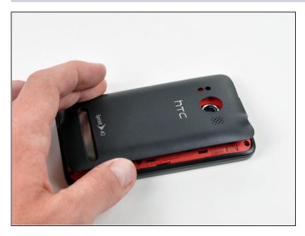
• Lift the rear panel off of the inner rear frame.
