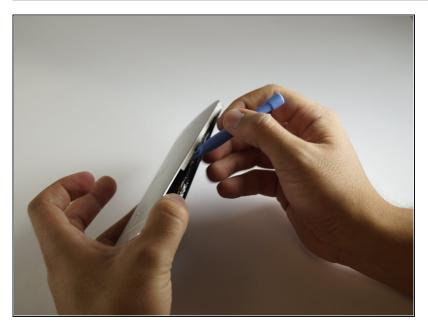
Gently remove the volume button. Using the plastic opening tool, loosen the back panel of the phone. Begin in the space where the battery was and work around the phone, following the crease of the back panel.
