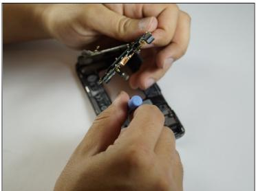
Lift the motherboard completely out of the phone. (may stay attached at the bottom by tape)
