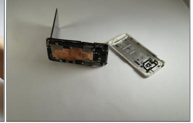
Pry the back open once loose and lift. The back panel will come off with time.
