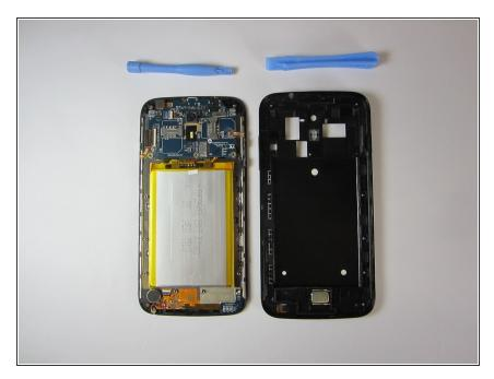
At this point your battery, motherboard, rear camera, and front camera should all be readily available for fixing. Happy fixing.
