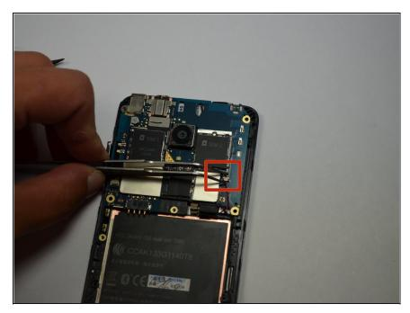
Using the <u>tweezers</u> gently disconnect the wire from the vibrator located on the motherboard.
