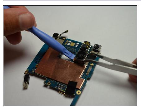
Carefully remove the ribbon that attaches the camera to the front screen using the <u>tweezers</u> and the plastic opening tool.
