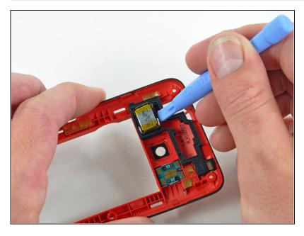
• Use an iPod opening tool to pry the rear speaker out of its housing in the rear inner frame.
