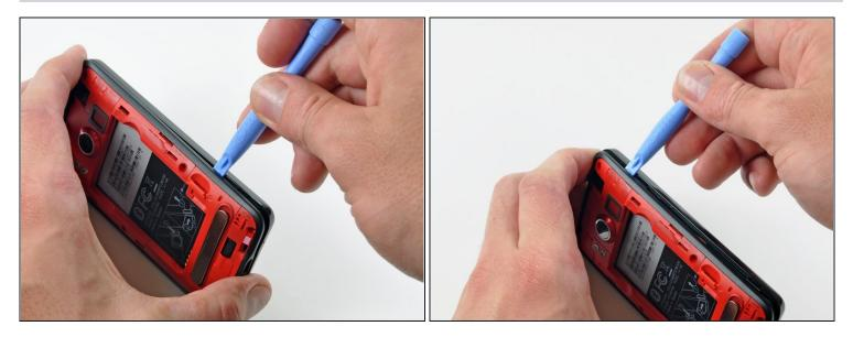
• Insert the iPod opening tool between the rear inner frame and its plastic surround and pry up at several points along the left edge of the Evo.
