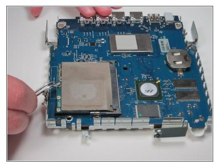
Unhook the wires connecting the logic board to the metal casing by grabbing and pulling up on each connection with tweezers.
