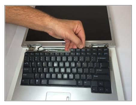
Gently lift the keyboard away from the laptop without harming the cord that is located at the bottom of the keyboard.
