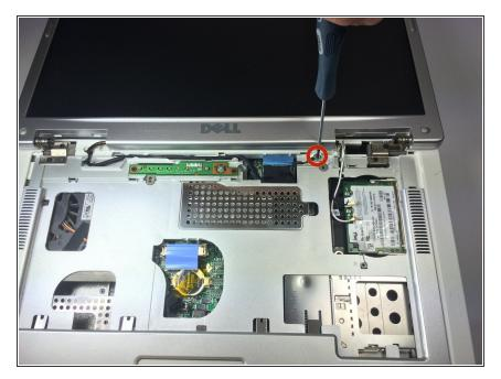
Remove one 4mm Philips #00 screw to completely disengage blue tab.
