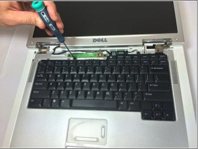
Remove two 4 mm Philips #00 screws.
