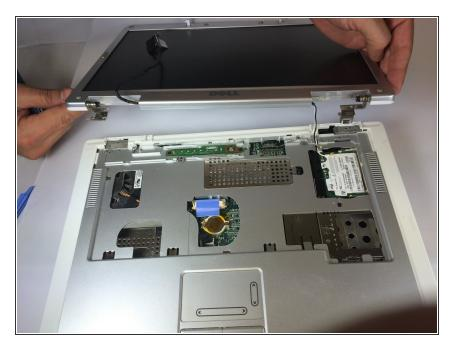
Separate the top panel of the laptop from the bottom panel.
