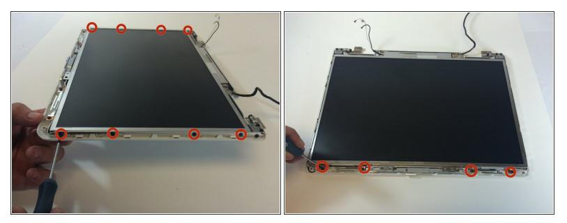
• Remove 12 4mm #00 Philips screws at the perimeter of the screen.
