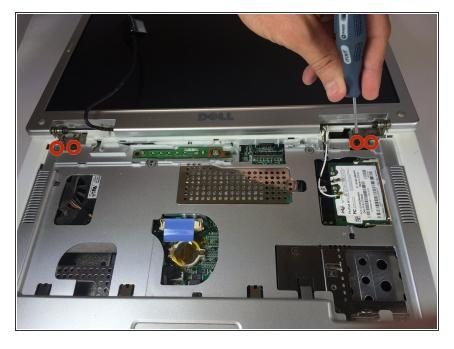
Remove four 4mm Philips #00 screws at the hinges for the screen.
