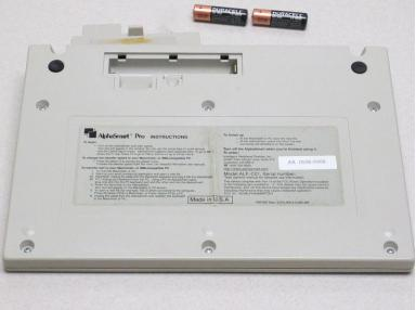
Remove each battery by using your fingers or the spudger to pry them from the compartment.
