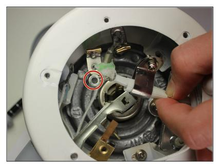
Locate another wire that is attached to the power cord and is covered by a thick layer of plastic, and is not ziptied to any other wires.
