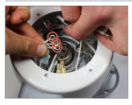
The remaining three wires are thin and not connected to the power cord or any other wires via ziptie.
