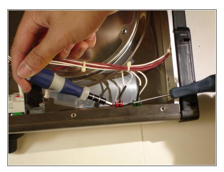
Using two thin screwdrivers (or similar objects) wedge them into the slots of the plastic shell of the desired light.
