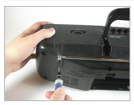
Loosen and remove the 8 mm screw using the #2 Phillips screw driver.
