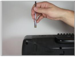
• Straighten the antenna to a vertical position and pull straight up (with a little force!) to remove the antenna.
