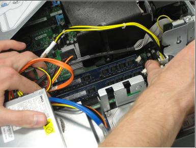
Press down on the white tabs on both sides of the RAM stick until the RAM stick pops up.
