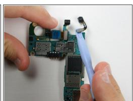
• Use a plastic opening tool or spudger to pry off the front-facing camera from the motherboard.
