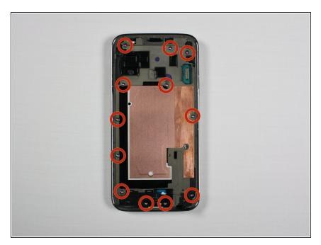
Remove the 12 4 mm Phillips screws #00 from the midframe.
