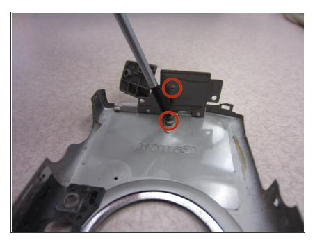
Unscrew two Phillips screws using a #00 Phillips screwdriver from front cover of the camera.
