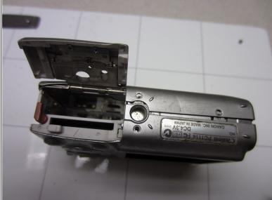
Slide the battery out of the battery compartment.
