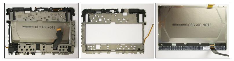
• Gently tear the LCD from its frame by lifting it from the tape connecting the two.
