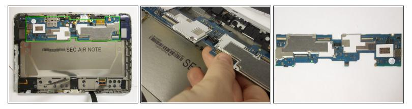
Once you have removed all the components connected to the motherboard, gently lift up on the area surrounding the green box and remove your motherboard.
